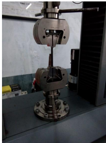
Figure 2. Sample of Resin+Carbon Fiber+Natural fiber on tensile testing machine
