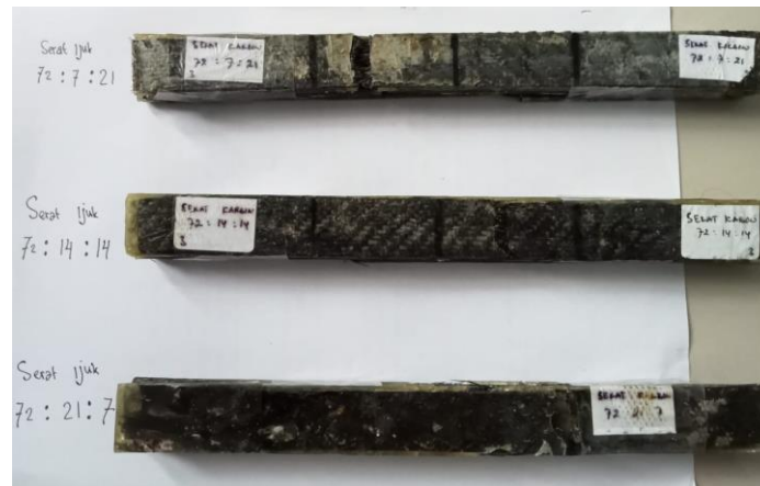
Figure 1. Carbon fiber/ ijuk fiber composite samples of B1, B2 and B3
